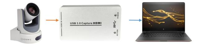
Use a high quality HDMI cable connect the source to the dongle.
