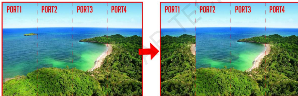
Figure 6-14 Left-right mirroring of the image loaded by Ethernet port 1
