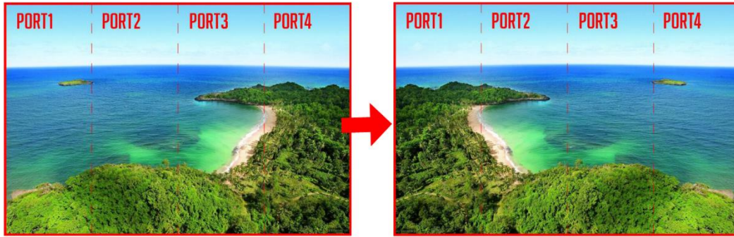
Figure 6-16 Left-right mirroring of the entire image
