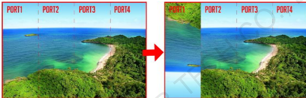
Figure 6-17 Top-bottom mirroring of the image loaded by Ethernet port 1
