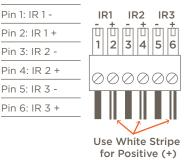
IR connections IR4 to IR6 (not shown in diagram) follow the same wiring as connections IR1 to IR3.
