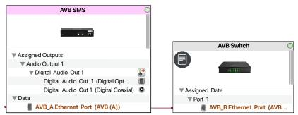
All Savant IP Audio devices in a multi-source AVB deployment of this type must be connected to the AVB switch via their Data/Ethernet ports as shown above.
