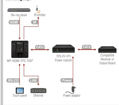
Connect the TPS output port of the transmitter to the TPS+PoE port of the TPS-PI-1P1 by a CATx cable.
