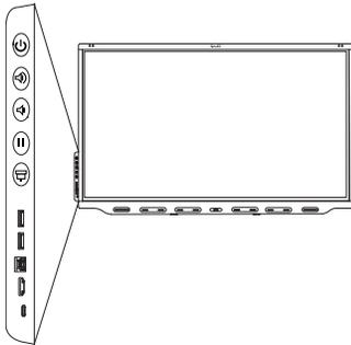
The convenience panel contains buttons for turning the display on and off, controlling the volume, freezing and unfreezing the screen, and showing and hiding a screen shade. It also includes connectors for USB peripherals and a computer or other input source.
