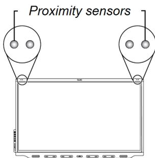
The proximity sensors are located in the top-left and top-right corners of the display's frame.
