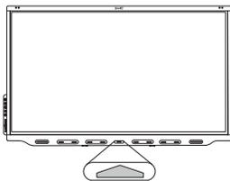
Tap the **Home** button on the display (pictured) or the remote control to open the Home screen (if iQ is enabled) or the Input screen (if iQ is disabled). From the Home screen, you can open the iQ apps, switch inputs, and adjust settings.
