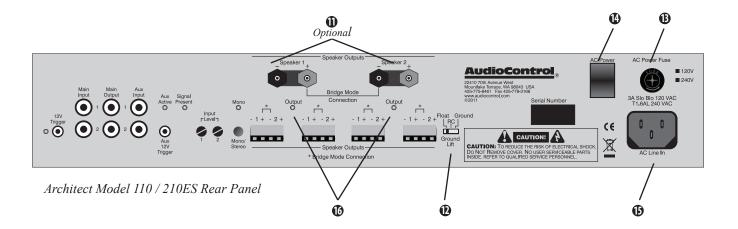
makes it very simple to pre-wire a system without ever taking the Architect out to the installation site. The two output blocks are paralleled to simplify connection to multiple speakers. The speaker connector blocks will accept up to 12 AWG wire.
