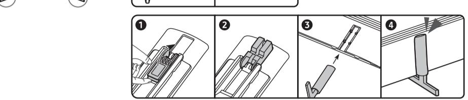
• Insert the Stands into the slot on the bottom of the TV.
