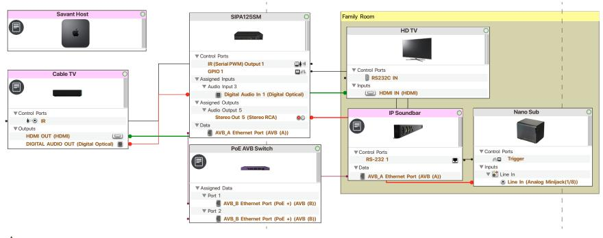
IMPORTANT! The above example shows the analog audio output of a PAV-SIPA125SM used in a speaker group. The analog output of a PAV-SIPA50SM cannot be used in AVB Speaker Grouping.
