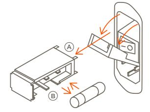
**Connection Pins Towards Unit** (A) B **Open Side of Cartridge Towards Power Switch**
