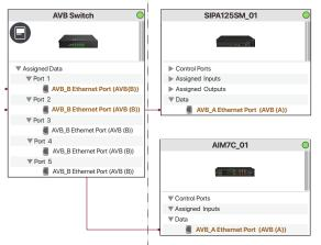
Savant IP Audio device Ethernet ports should be connected to ports on the AVB switch as shown in the example image.
