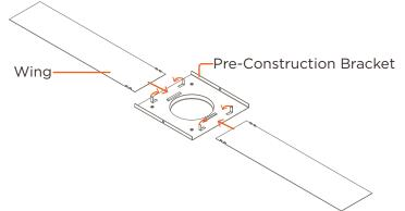
Once in place, fold tabs on pre-construction bracket down (x4).
