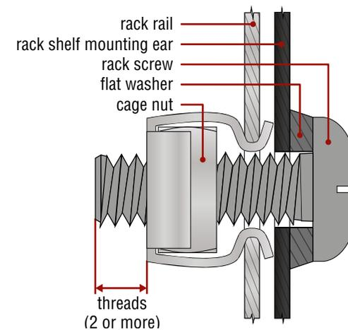
**ATTENTION!** Fix the frame to the rack rail by applying all mounting holes. Choose properly sized screws for mounting. Keep minimum two threads left after the nut screw.
