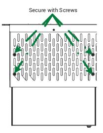
Install the blanking plate (if required) using the provided screws
