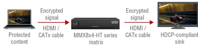
All the devices are HDCP-compliant, no manual setting is required, both protected and unprotected contents are transmitted and displayed on the sink.
